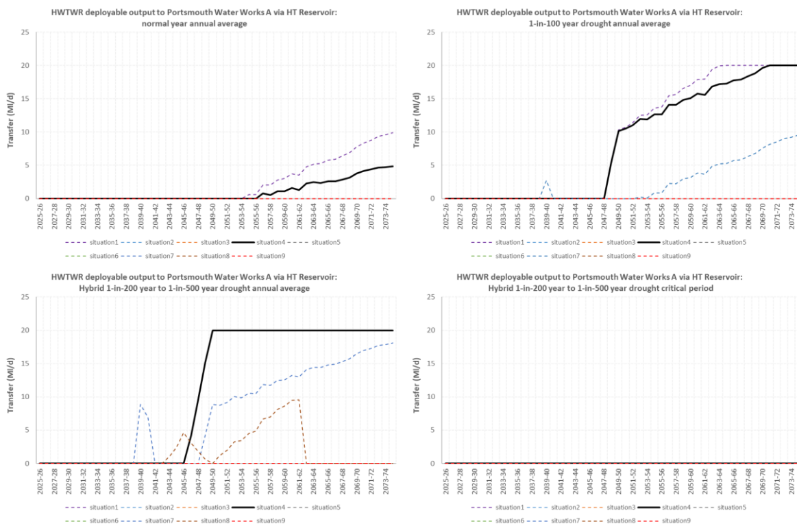
Figure 13: Utilisation of the raw water transfer from HWTWRP to Portsmouth Water Works A via Havant Thicket Reservoir.
