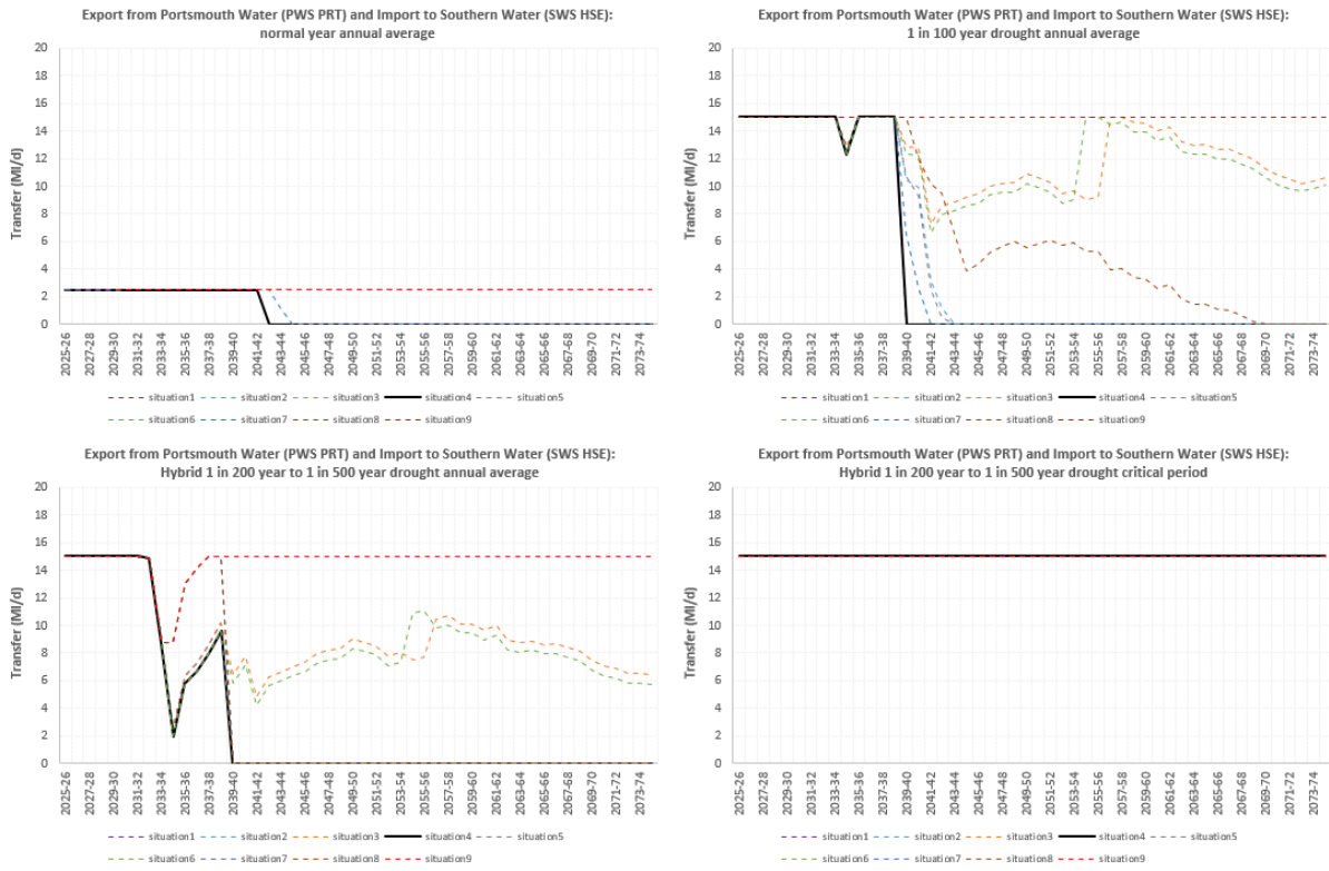
Figure 15 Modelled utilisation of the 15 MI/d capacity export from Portsmouth Water to Southern Water’s HSE WRZ (sensitivity test with 2.5 MI/d cap on normal year export)
