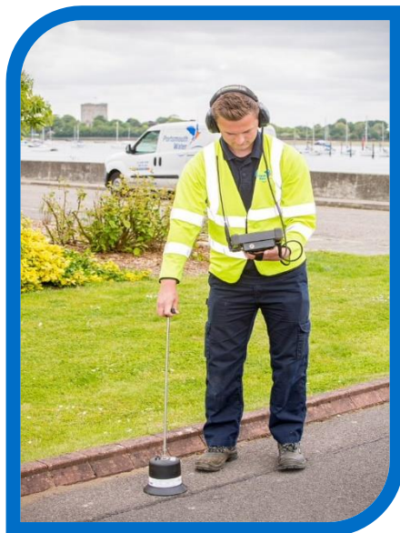
Figure 5 - one of our team out detecting leaks
